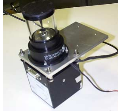
Figure 2: The omnidirectional camera and accelerometer setup
